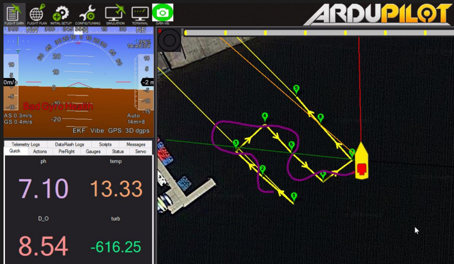
Example monitoring in ArduPilot
