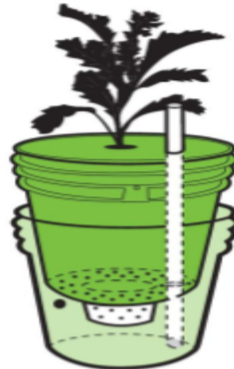
Figure 4; the drip system where the plant nutrients are dripped slowly into the top basin
