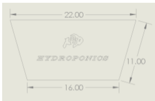
Figure 10 ; the drawing for the larger side piece of the wooden housing
